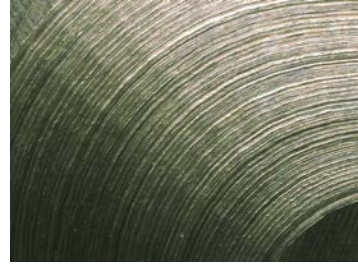
Figure 3: A macro image 10:1 of the “sealing groove”
