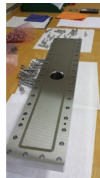
Figure 4: A special vacuum test adapter for all principle tests and for the final acceptance test like rest gas analysis and leak check.
